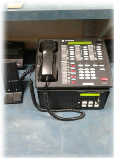
Back up radio/dispatch console at Fire Station #1
