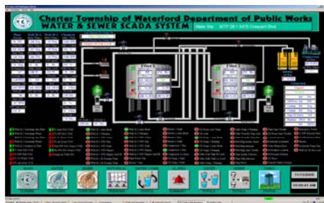
Screen Shot of the DPW's Supervisory and Control And Data Acquisition System (SCADA). The DPW electronically monitors and alarms on over 1,200 variables.
