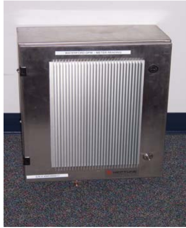
Neptune R-450 Fixed Network Collector. These collectors receive daily meter reads and then transmit the data to the DPW using the Township's Broadband Wireless System.
