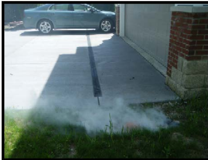
4755 Motorway (alt view 1), Smoke from drainage area and slot drain along driveway.
