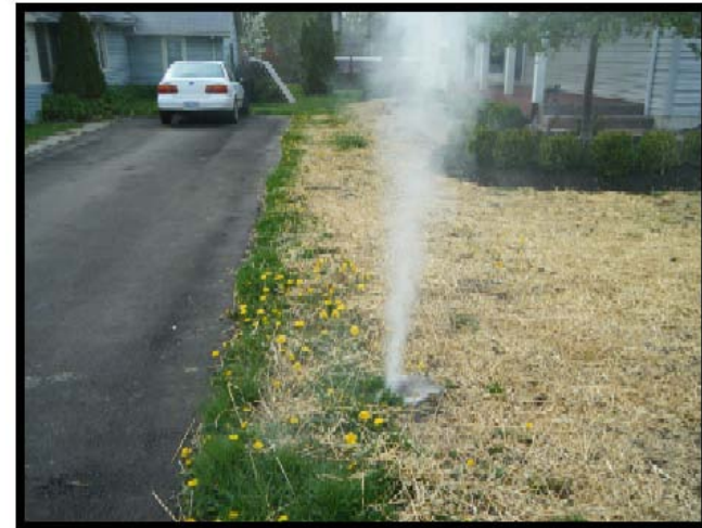
1440 Otter, Smoke from cracked clean out.
