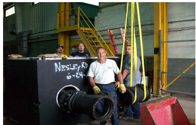
DPW Distribution Crew fabricating Booster Station Vault at the DPW Yard
