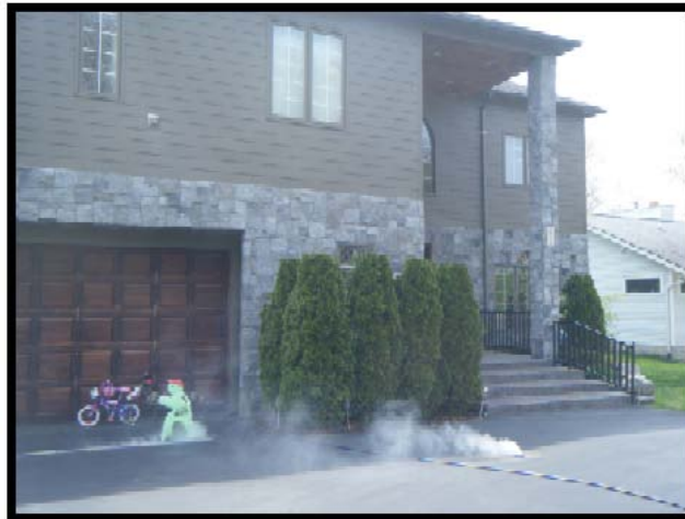
1053 Stratton, Smoke from slot drain & clean out. (Drains entire driveway)
