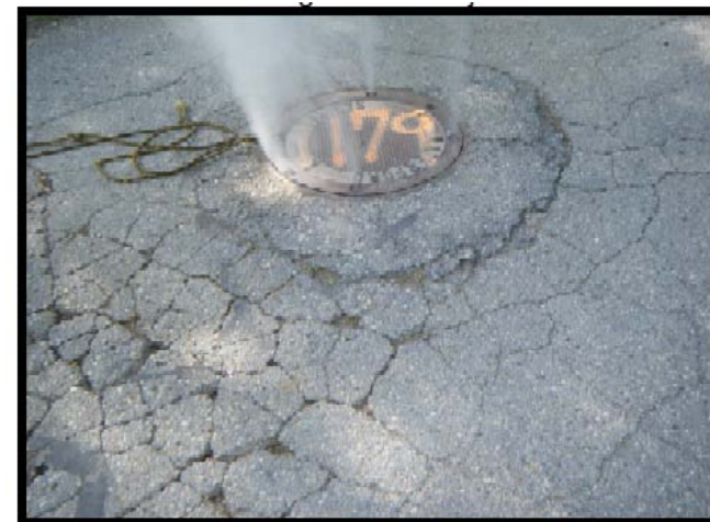
MH#1179, Smoking from cracks in asphalt and around rim, needs bolt hole plugs.
