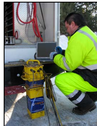
Joe Ashley Performing Flow Meter Maintenance
