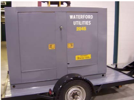
A portable generator used by the DPW during power failures. These are used at sites without permanent stationary generators.
