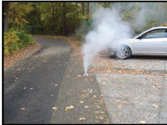
3848 Cottage Grove, smoke coming out of cleanout, cap missing
