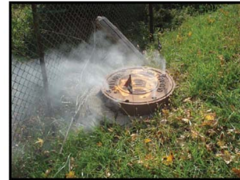
Smoke through bolt holes and around flange. Low lying area. Resident confirms flooding in spring.
