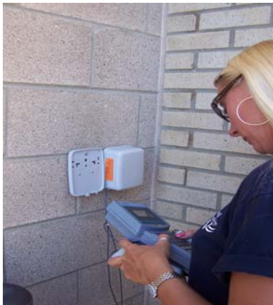
Service Branch employee Penny Holden configuring R-450 Reading Devices in the Field.
